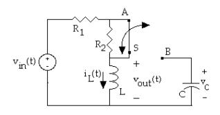
a. For  $0 \le t < 10$ , Determine the system transfer function. (2 pts)
